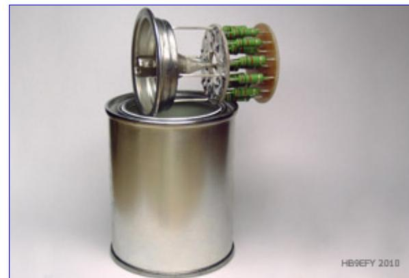
[02] load resistor and RF-proof metal can
